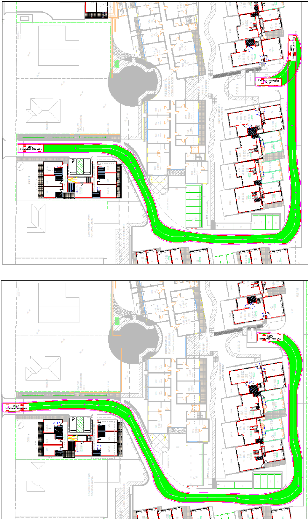
Figure 10 Swept Paths for service vehicle (MRV) Waste Collections Area 1 Source: Based on plans provided by Edmiston Jones and using Autoturn tool
